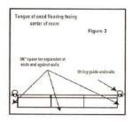
Leave a ¾" expansion gap at each end. Set nails and fill holes with matching putty. Remove string and nails.
