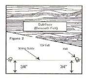
**Note:** This dimension should be 4" when installing 3  $\frac{1}{4}$ " wide flooring. When a room is greater than 20 ft. in width, the direction of the installation should start near the center of the room and work out towards the walls placing a loose spline where the two grooves come together.
