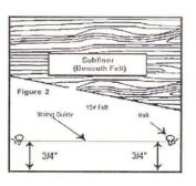
**Note:** This dimension should be 4" when installing 3  $\frac{1}{4}$ " wide flooring. When a room is greater than 20 ft. in width, the direction of the installation should start near the center of the room and work out towards the walls placing a loose spline where the two grooves come together.
